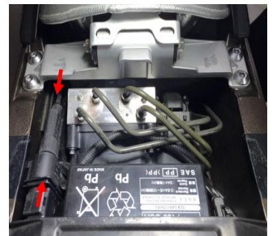
Fig4. Installed Active Tune Lamda Controller
